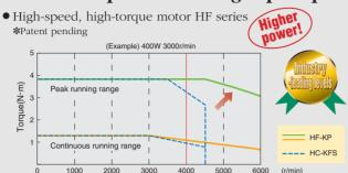
The high speed motors (6000r/min) and high speed frequency response amplifiers (900Hz) shorten positioning times.
