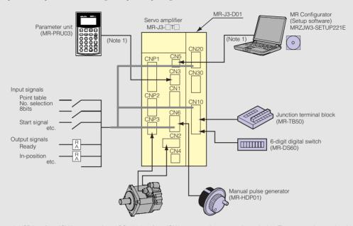
Notes: 1. USB interface (CN5 connector) and RS-422 interface (CN3 connector) are mutually exclusive. They cannot be used at the same time. 2. MR-J3-D01 is not available with the indexer function.
