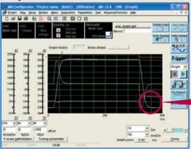
Powerful graph functions with 3 analog channels and 4 digital channels support tuning. User-friendly functions such as [Over write] and [Graph history] and a diverse waveform selection powerfully support user's work. Also, the [Gray display] function is provided for easy reading of printed data. Data can be saved either in CSV or JPEG format.
