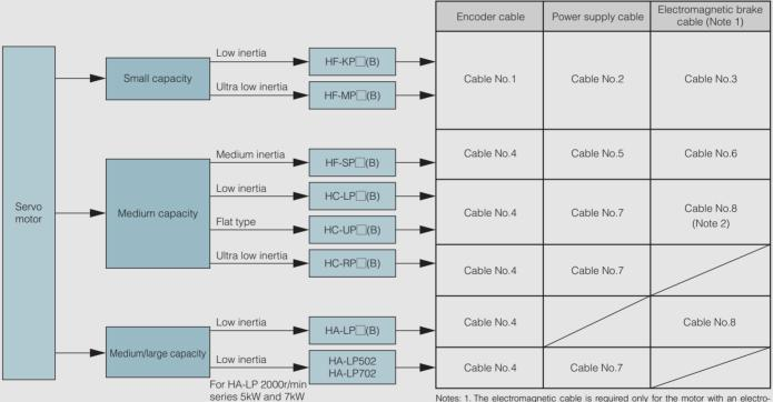
Notes: 1. The electromagnetic cable is required only for the motor with an electromagnetic brake.
