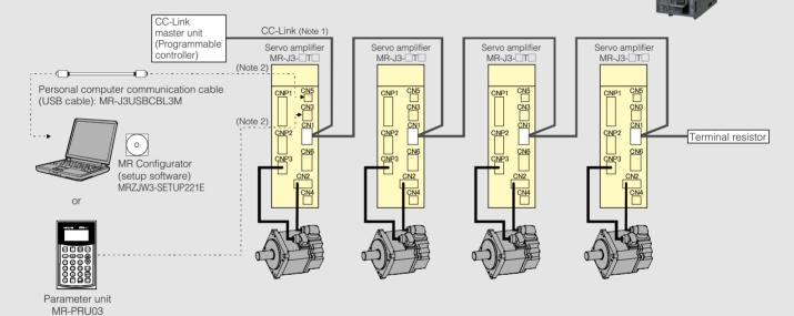
Notes: 1. When using only remote device stations, up to 42 servo amplifiers can be connected when 1 station is occupied by 1 servo amplifier, and up to 32 servo amplifiers when 2 stations are occupied by 1 servo amplifier.
