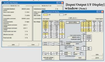
The [Input/Output I/F Display] window has been renewed. The [Input/Output I/F Display] window and [Amplifier Data Display] window can be displayed simultaneously, so the DI/DO ON/OFF status and operation status can be checked in real time.
