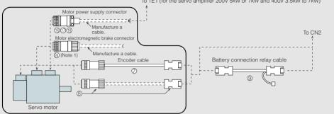
Notes: 1. The electromagnetic cable is not required for 1.5kW or smaller servo motors of HC-LP series and of HC-UP series as the power supply connector has electromagnetic brake terminals
