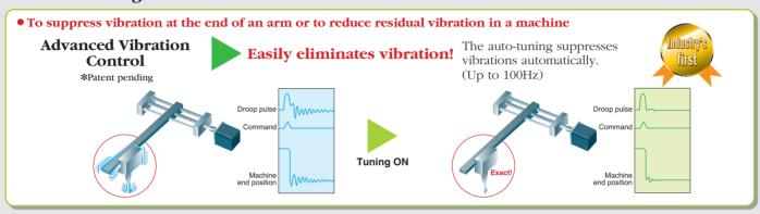
• To suppress drive shaft vibrations such as in a ball screw
