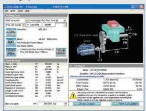
A user-friendly design facilitates selecting the optimum servo amplifier, servo motor (including the servo motor with an electromagnetic brake) and optional regeneration unit just by entering constants and an operation pattern into machine-specific windows.
