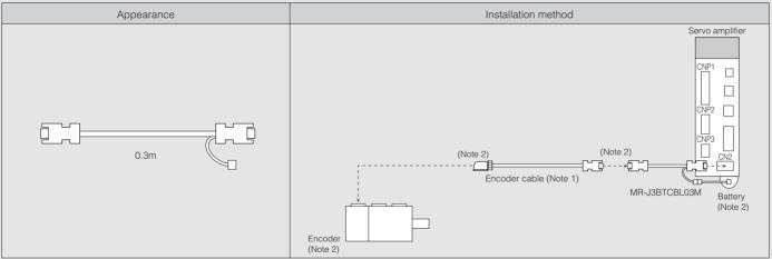
Notes: 1. The encoder cable varies depending on the motor series. Refer to the section "Options ● Cables and connectors" in this catalog 2. To hold the absolute value, the encoder, the encoder cable (s), the relay cable and the battery must be kept connected.
