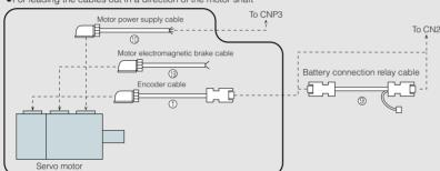
• For leading the cables out in an opposite direction of the motor shaft
