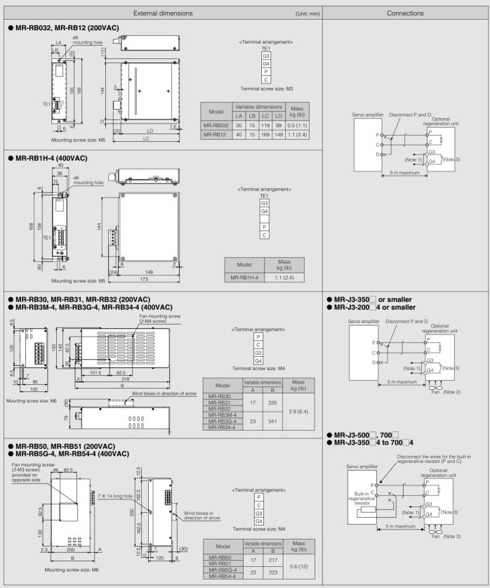
Notes: 1. Create a sequence that turns off the magnetic contactor (MC) when abnormal overheating occurs.
