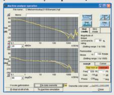
When the [Start] button is pressed, the servo motor is automatically oscillated, and the machine system's frequency characteristics are displayed.
