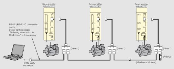
Notes: 1. Branch connector, BMJ-8 (HACHIKO ELECTRIC CO., LTD) is recommended. Refer to the section "Ordering Information for Customers" in this catalog. 2. Connect a terminal resistor, 150Ω.
