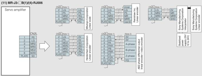
Notes: 1. When manufacturing the linear encoder connection cable, use the optional CN2L connector (MR-J3CN2). Refer to "MR-J3-B-RJ006 SERVO AMPLIFIER INSTRUCTION MANUAL" for details on the wiring
