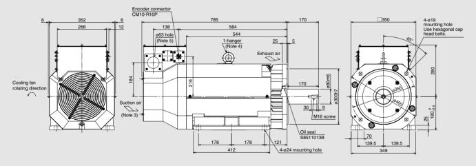
\* The terminal block on the terminal box housing consists of M10 screws for the motor power supply (U, V, W), and M4 screws for the cooling fan (BU, BV, BW) and for the thermal protector (OHS1, OHS2).
