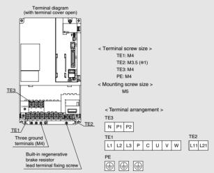
\*1. The TE2 terminal screw size has been changed to M3.5 from April 2007. For the servo amplifiers manufactured on or before March 2007, the terminal screw size is M3.
