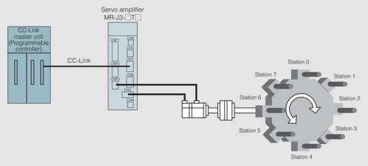
Notes: 1. Servo amplifier with software version A4 or above is required for the indexer function.
